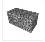
Gabions are wire mesh baskets formed by connecting individual panels of mesh with helical spirals on the vertical edge wires creating an open series of box compartments that fold in a concertina fashion to be flat packed.
