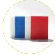
Polyethylene sheets with double coloured layer (sandwich panels)
