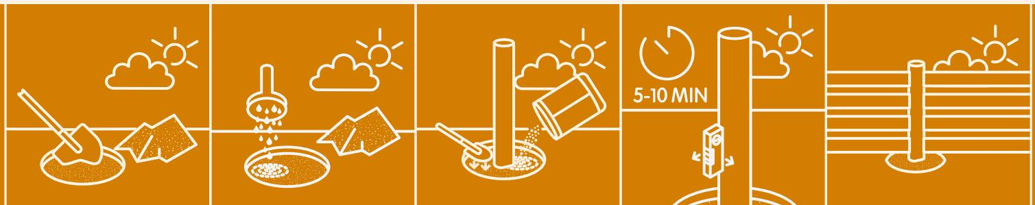
any remaining water on the concrete. The concrete hardens quickly, bracing is not necessary. Smooth the surface or cover it with soil or turf.
